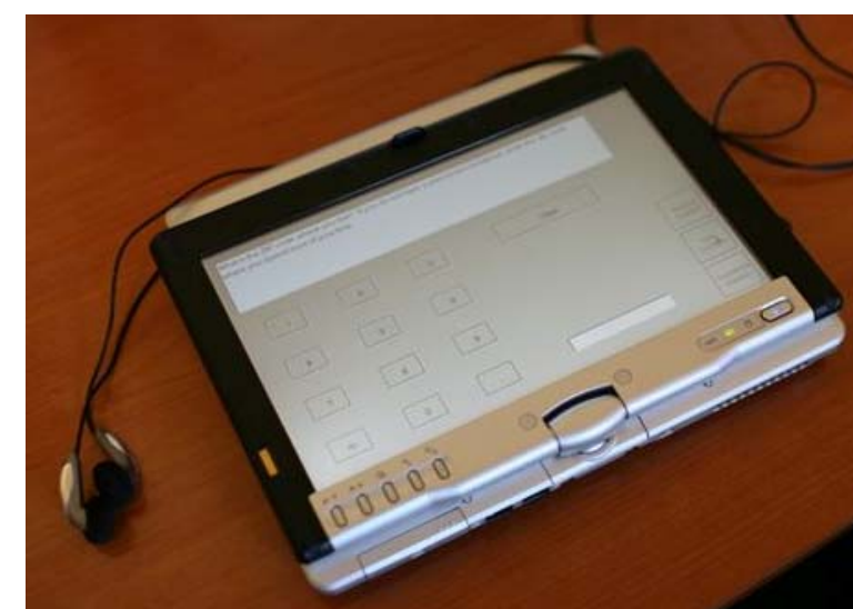
7-inch touchscreen with audio, for a visually impaired or illiterate client
